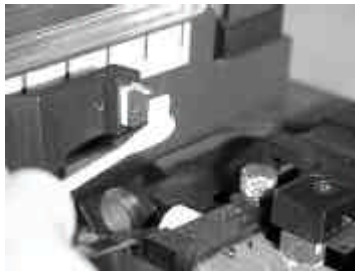
Figure 53. Cleaning the Bare Fiber Pads
