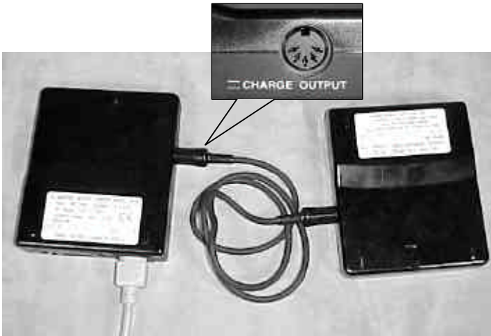
Figure 8b. Battery Installation
