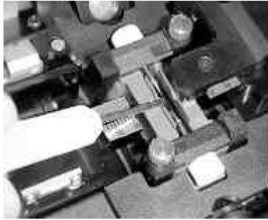
Figure 52. Cleaning the V-Grooves
